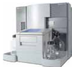
SPR (Surface Plasmon Resonance) analyzer Test Method : Binding affinity Test
